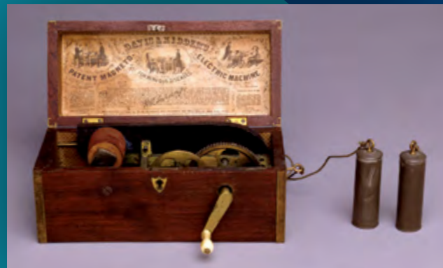
Early electric stimulation machine. Davis & Kidder's "Patent Magneto-Electric Machine" manufactured by W. H. Burnap, ca. 1854.
